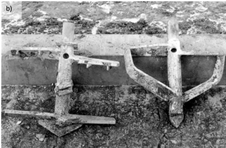
Figure 1: (a) Typical machinery for manufacturing lime-cement columns (b) Pin drill and Swedish standard mixing tool (courtesy of Skanska AB; Larsson et al. 2005).
