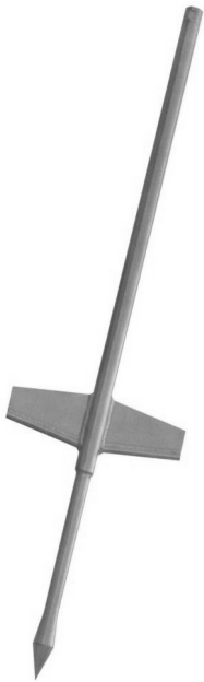
Figure 2: The column penetration test ( KPS ) (courtesy of Geotech).
